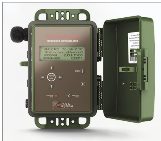
Figure 23. Acoustic monitoring devices for detecting coqui frogs
